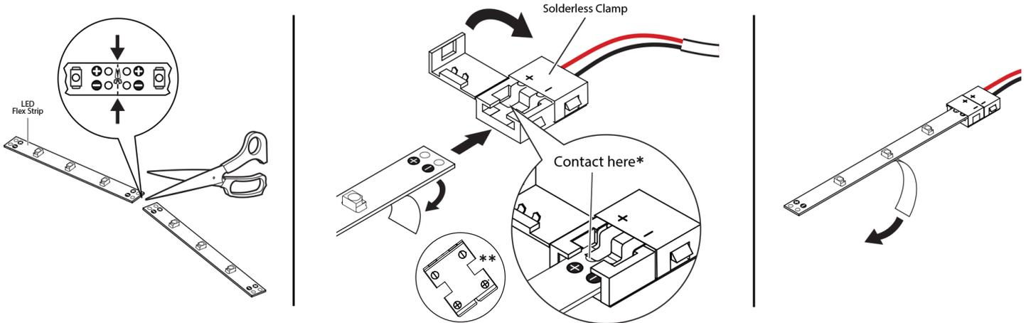
1. Cut the tape light at a cut point (marked by a dashed line) between two pairs of positive and negative connection points.
